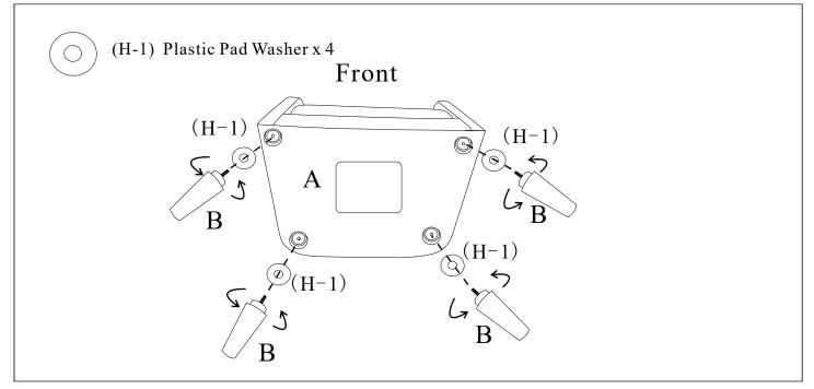
Place Seat (A) on it's back onto a padded, non-marring surface. Unzip cover and remove the leg packaging from the interior. Insert Legs (B) with Plastic Pad Washer (H-1) into position, staking the components in the order as shown. Turn Legs (B) clockwise until fully tightened. Do not over tighten. Re-zip cover.
